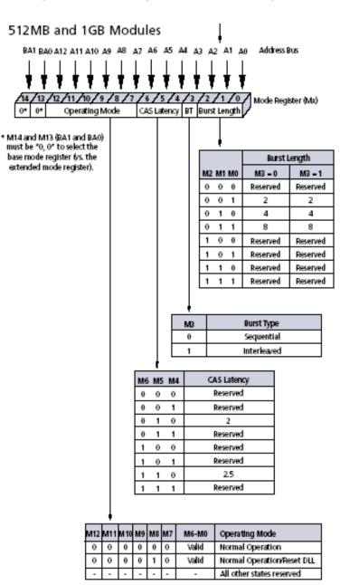
Figure 4: Mode Register Definition Diagram
